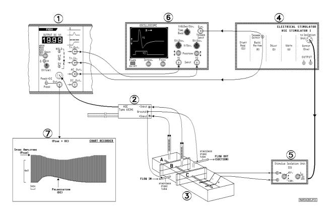
Fig. 3: Typical experimental set-up for measurement with the PHDA. For description see text.
