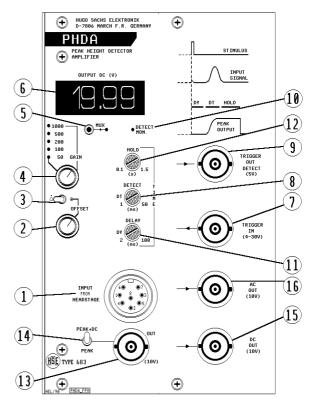
Fig. 6: Controls and indications on the front panel.
