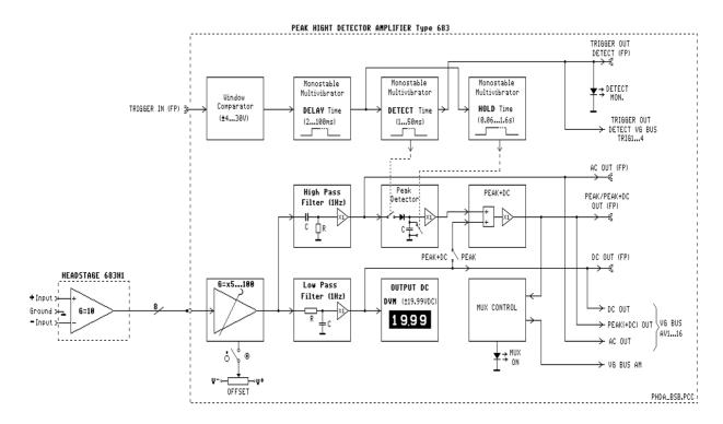
Fig. 5: Block diagram oft the Peak Height Detector Amplifier PHDA
