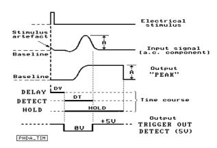
**Fig. 4**: Time course during capture of the peak amplitudes.Note: negative signals are not recorded.
