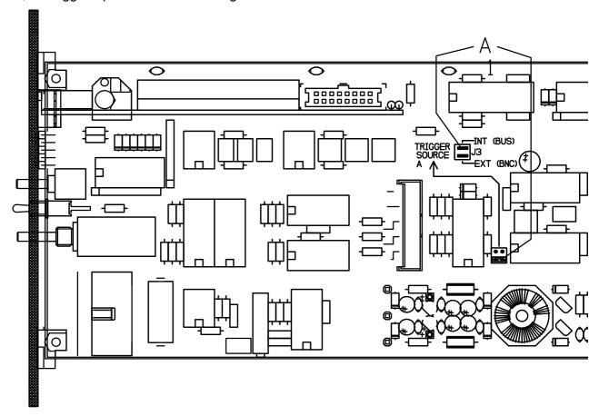
**Fig. 8**: View of circuit board of the PHDA. Before installing the module in the housing the links A...D have to be determined. Note details in the text!
